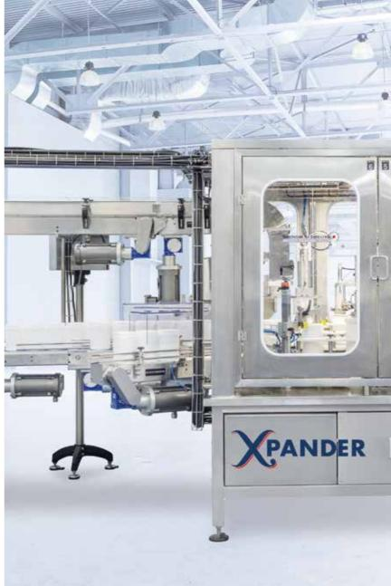
"Designed for operational flexibility and ultra-low, tools-free, sub 40-minute format parts changeover, it offers advanced Quality Control including multiple check-weighers and total QC for sealing and capping, significantly increasing efficiency."
