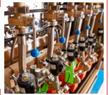
FDA-approved pipes and piping works, screw-less engineering and tri-clamps fittings
