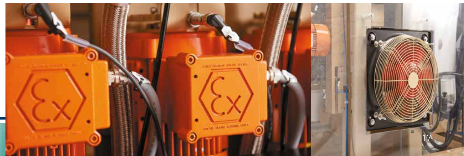
SHEMESH AUTOMATION'S FGW-120 FILLING MACHINE WITH COMPLETE EXPLOSION (EX) AND CORROSION PROTECTION
