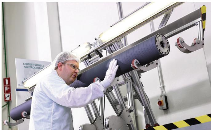
CFRP is becoming the material of choice for many applications in the nonwovens industry. Why? Critically, CFRP offers significantly reduced deflection over rollers made from other materials like steel and aluminum. This enables the use of much longer rollers, which in turn brings greater efficiency and larger scale to production, enabling greater sizes and faster speeds.
